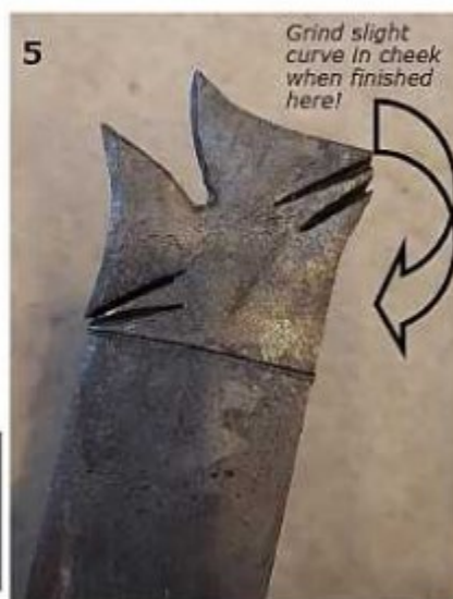
1. Finished Fox! 2. Marking material. 3. Layout of face. 4. Eye punch is shaped like a football. Note: Cheeks are ground slightly to give personality to fox. 5. Layout cuts on bar. Easier to work with bar attached, then cut off when necessary. 6. Tool made for creating cheek depressions.
